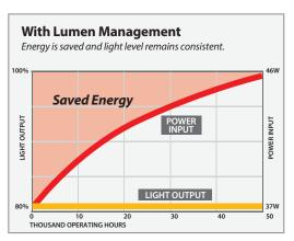
With nlight 80% lumen management input watts start at 37 and gradually increasing to 46 at 50,000 hrs when using 48L system.
