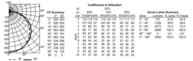
2BZL2 34L LP835 EZ1, 3672 delivered lumens, test no. LTL25223P, tested in accordance to IESNA LM-79.
