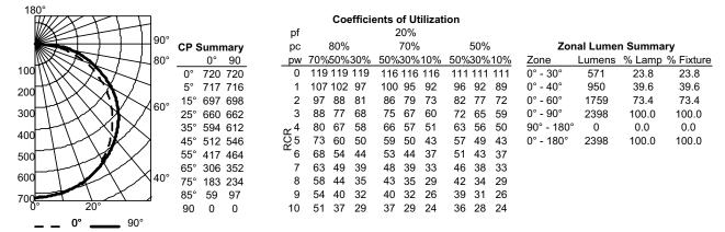
2BZL2 30L EZ1 LP835, 3098 delivered lumens, test no. LTL 24736P3, tested in accordance to IESNA LM-79.
