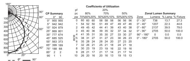
2AVL2 40L MDR LP835, 3806 delivered lumens, test no. 69075P9, tested in accordance to IESNA-LM79.
