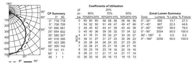
2AVL2 30L MDR LP835, 2704 delivered lumens, test no. 69075P5, tested in accordance to IESNA-LM79.
