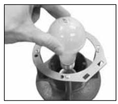
4. Install lamp of proper type and wattage shown on fixture label & chart on page 2. Do not exceed maximum wattage.
