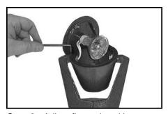
**Step 6 -** Adjust fixture head into selected orientation and tighten setscrew using <sup>5</sup>/<sub>64</sub>" allen wrench. Coat cap screws with silicone grease and install cap.
