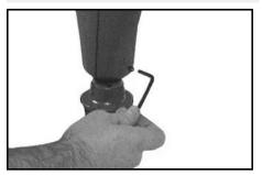
**Step 5 -** Loosen setscrew, adjust fixture rotation, and tighten setscrew.
