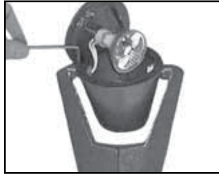
Step 6 - Loosen screw, adjust fixture angle and tighten screw. Coat cap screws with silicone grease and install cap.
