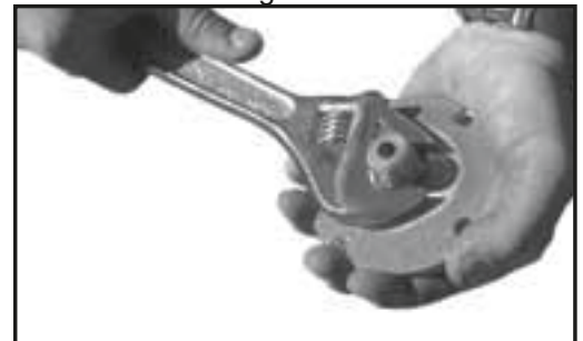
Step 2 - Tighten coupling onto mounting device. (Consult KIM Landscape Catalog for mounting device options.)
