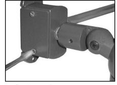
7. Replace splice compartment cover and gasket.
