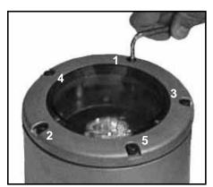
10. Make sure gasket surface is clean and free of all dirt and debris so a leak free installation can be achieved. Replace lens, gasket and lens ring. Secure with allen head cap screws (5). Tighten opposing screws progressively and evenly to 20 inch/pounds, (1.67 ft. lbs.).
