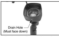
7. Replace lens (convex side out) fitting lens gasket assembly into the recess on fixture body. Replace light shield over lens after making sure the drain hole is down, so water will not stand on lens. Tighten opposing screws progressively and evenly.
