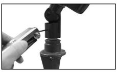
8. Loosen set screw, adjust fixture rotation, and tighten set screw.
