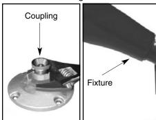
2. Tighten coupling onto mounting device. (Consult KIM Landscape Catalog for mounting device options.) Install fixture onto coupling.
