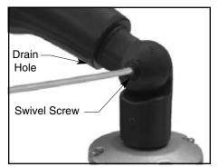
6. To adjust angle loosen swivel screw and position fixture at selected angle. Tighten swivel screw firmly. Caution: Drain hole must be aimed down after installation is complete.
