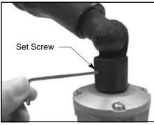
5. Loosen set screw, adjust fixture position and tighten setscrew.
