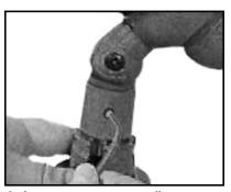
Loosen setscrew, adjust fixture rotation, and tighten setscrew.
