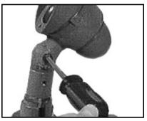
5. Loosen screw, adjust fixture angle, and tighten screw.
