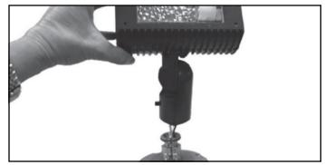
2. Attach fixture onto coupling.
