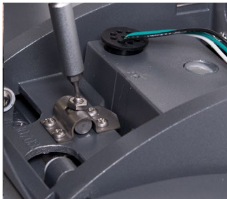
17. Loosen or tighten set screw to adjust tilt (+10° (away from the wall) and -5° (towards the wall)).
