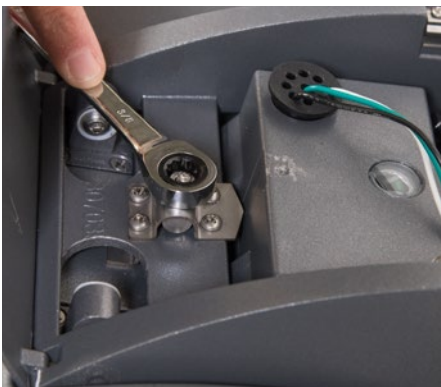
16. Loosen the nut to allow for tilt.
