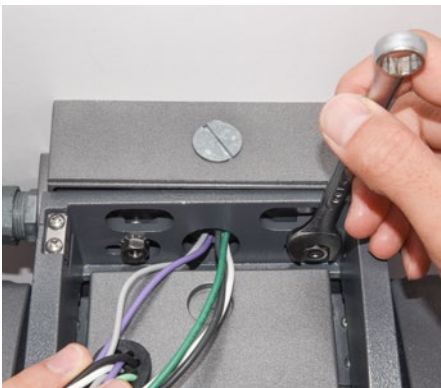
13. Hold fixture with both hands, and guide keyhole slots on back of fixture housing onto mounting back plate studs/nuts. Using wrench, secure fixture by tightening nuts inside housing.
