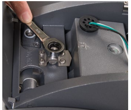
18. Tighten nut to lock in the tilt.
