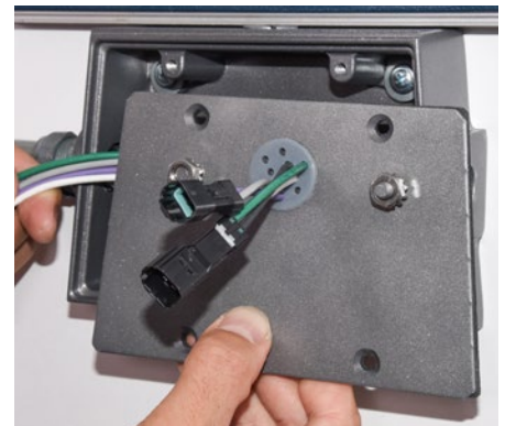
6. Install the Rubber Grommet into the Mounting Bracket with the Wire Connector facing outwards. Loosely Screw the 2x Locknut on the Mounting Bracket
