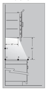
**Over Cabinets** Trac 12, using Tl214LED-27K-WD modules spaced 6" on-center, generally provides excellent indirect lighting. Placing the fixture at the front edge of the cabinet top will project light into the space and illuminate any displayed objects. Locate top of lamp even with top edge of cove molding to prevent a harsh shadow line.
