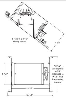
Mounting Frame 22-gauge die-formed galvanized steel mounting frame ● Rough-in section (junction box, mounting frame, housing and bar hangers) fully assembled for ease of installation.
