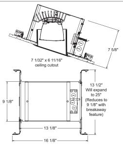
**Junction Box** Pre-wired junction box provided with (5)  $\frac{1}{2}$ " and (1)  $\frac{3}{4}$ " knockouts, (4) non-metallic sheathed cable connectors and ground wire, UL and cUL listed for through-branch wiring, maximum 8 No. 12 AWG 90° C branch circuit conductors (4 in, 4 out) • Junction box provided with removable access plates • Knockouts equipped with pryout slots • Push-in electrical connectors supplied as standard for fast, secure installation.
