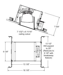
Junction Box Pre-wired junction box provided with (5) ½" and (1) ¾" knockouts, (4) non-metallic sheathed cable connectors and ground wire, UL and cUL listed for through-branch wiring, maximum 8 No. 12 AWG 90° C branch circuit conductors (4 in, 4 out) • Junction box provided with removable access plates • Knockouts equipped with pryout slots • Push-in electrical connectors supplied as standard for fast, secure installation.
