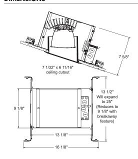
**Junction Box** Pre-wired junction box provided with (5) ½" and (1) ¾" knockouts, (4) non-metallic sheathed cable connectors and ground wire, UL and cUL listed for through-branch wiring, maximum 8 No. 12 AWG 90° C branch circuit conductors (4 in, 4 out) • Junction box provided with removable access plates • Knockouts equipped with pryout slots • Push-in electrical connectors supplied as standard for fast, secure installation.
