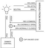
The Dimming Relay Leads can be used to accommodate a 0-10V dimming signal, allowing the load to operate at the desired dimmed setting, but enabling the inverter to bypass the dimmed state and operate the load at full brightness while in the emergency mode.
