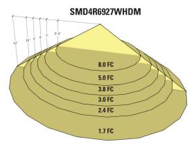
DD = distance down to illuminated work plane FC = initial foot-candles at nadir
