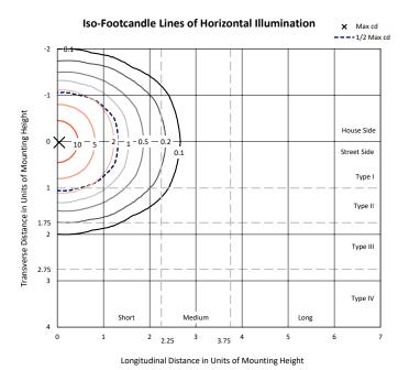
Based on 10 foot mounting height. Maximum calculated value = 14.8 fc Type V - Short - Full Cutoff
