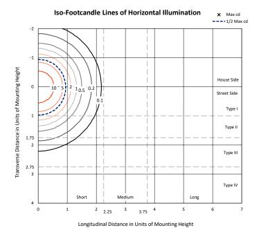
Based on 10 foot mounting height. Maximum calculated value = 18.7 fc Type V - Short - Full Cutoff
