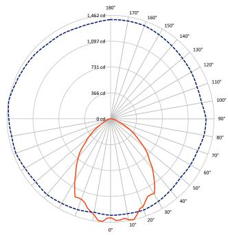
Vertical Plane Through 260-Deg Lateral ---- Horizontal Cone Through 12.5-Deg Vertical
