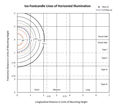
Based on 10 foot mounting height. Maximum calculated value = 14.7 fc Type V - Short - Full Cutoff
