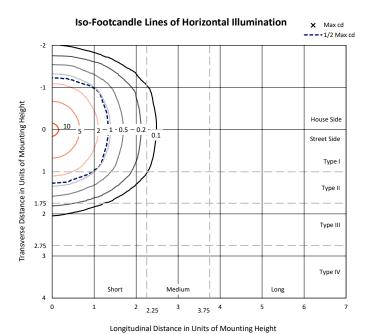
Based on 10 foot mounting height. Maximum calculated value = 10.6 fc  $$\operatorname{\sc Type}$$  II - Short - Cutoff
