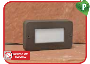
SL17ALLEDPWBR: NO BACK BOX REQUIRED 12v Driver Supplied Cast aluminum or brass 12v 4w integrated flat panel LED 50,000 hours average rating 3000K warm white or 5200K cool white External 12v AC driver required (supplied)
