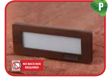
SL08ALLEDPBAR: NO BACK BOX REQUIRED 12v Driver Supplied Cast aluminum or brass 12v 8w integrated flat panel LED 50,000 hours average rating 3000K warm white or 5200K cool white External 12v AC driver required (supplied)
