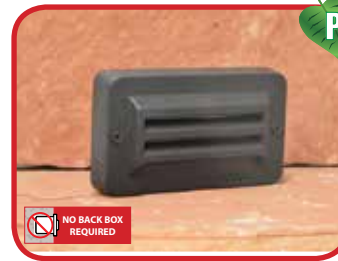
SL17LEDPBLT: NO BACK BOX REQUIRED 12v Driver Supplied Cast aluminum or brass 12v 4w integrated flat panel LED 50,000 hours average rating 3000K warm white or 5200K cool white External 12v AC driver required (supplied)
