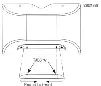
1.Slide tabs "A" between housing and lens gasket.
