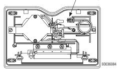
Attach unit cover to backplate by reversing Step 1. Ensure all wires are within enclosure to avoid pinching with cover.
