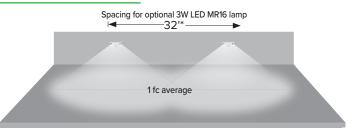
Meets Life Safety Code minimum illuminance of 0.1 fc and average illuminance of 1.0 fc. Assumes open space with no obstructions, mounting height of 7.5', ceiling height of 9' and reflectances of 80/50/20 on a 3' path. Photometry files available on the Dual-Lite web site.
