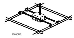
Use template provided to cut hole in ceiling tile. (Note the range of hanger bars - template should be centered along hanger bar direction.) Knock out the most convenient knock-out in the enclosure and thread wiring through, and install conduit fitting and conduit. Mount hanger bars with clips to the T-Grid. Slide the trim ring down to level of tile face and tighten trim ring screws.
