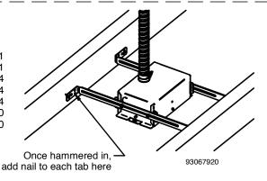
Remove the hanger bar screws on the sides of the enclosure and slide the hanger bars out of the tabs.
