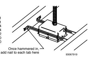
Use template provided to cut hole in ceiling. (Note the range of hanger bars - template should be centered along hanger bar direction.) Knock out the most convenient knock-out in the enclosure and thread wiring through, and install conduit fitting and conduit. Hammer hanger bars into joists and secure with one nail through one hole in each hanger bar . Slide the trim ring flush with theceiling face and tighten trim ring screws.
