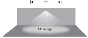
Meets Life Safety Code minimum illuminance of 0.1 fc and average illuminance of 1.0 fc. Assumes open space with no obstructions, mounting height of 7.5', ceiling height of 9' and reflectances of 80/50/20. Photometry files available on the Dual-Lite web site (www.dual-lite.com).
