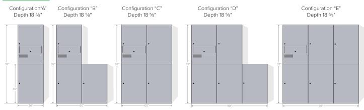
Consult factory for alternate runtimes and battery cabinet configurations. External transformer (not illustrated) is provided for 12.5K and 15.0K configurations with 208VAC and 240VAC input. Transformer cabinet dimensions are 18" W x 28" H x 15" D and weighs 250 lbs.
