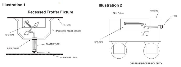
NOTE: MARK AN APPROPRIATE LABEL ON INDICATOR LIGHT AND TEST SWITCH AFTER INSTALLATION.
