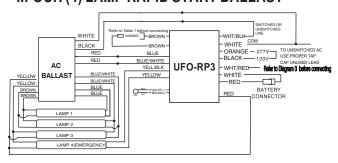
NOTE: Use the proper input voltage lead, cap unused lead
