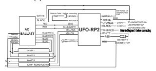
NOTE: Use the proper input voltage lead, cap unused lead
