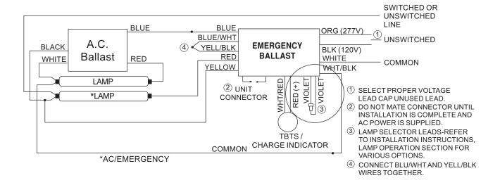
This unit can be used with most 2'-4' lamps. Refer to the chart below for the type of lamp(s) operated and the number of lamps to be operated in emergency mode.
