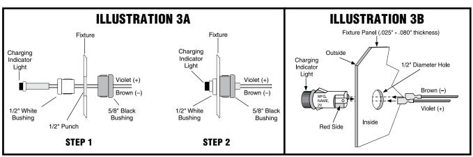
NOTE: After installing the charging indicator light and test switch, mark each with the appropriate label. If a detached charging indicator light is used, connect by matching wire colors and install as shown on the installation insert page.
