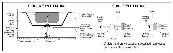
NOTE: After installing the charging indicator light and test switch, mark each with the appropriate label.
