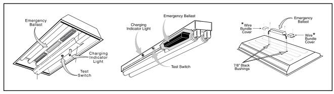
\*For installation on top of the fixture, wire bundle covers may be required by state or local codes. These covers are available from the manufacturer as an accessory kit and must be ordered separately. Call your local distributor or the factory for complete infomation.
