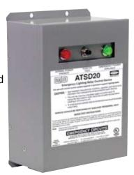
The ATSD20 is compatible with all lamp types. However it is not recommended for use with HID lamps. The time to achieve full HID illumination when transferring to emergency power from an "off" switch position under emergency conditions may not meet NFPA 101 requirements.
