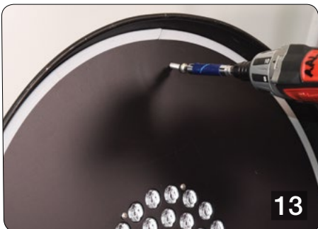
Using new 1/4-20 Screws and O-rings, attach new deck assembly to housing. Torque screws to 48 in lbs.
