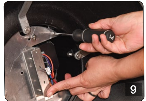
Install new driver assembly back and secure in place using provided screws (hand tighten).
