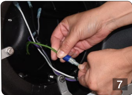
Connect wires from new driver assembly, Make sure to follow wire polarity i.e. green to green, white to white etc. Tuck leads into driver housing (make sure not to pinch wires).
