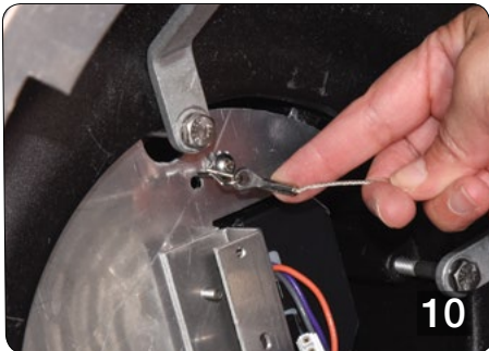
Attached (2) safety cables from new Deck Assembly. As shown.
