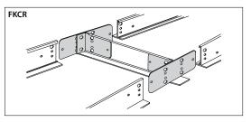
For flanged fixtures in row configurations, the FKCR adapter bracket kit is required in addition to the FK14 kit. Order one less FKCR than the total number of fixtures in row. (Example: Row of two, order (2) FK14 & (1) FKCR)
