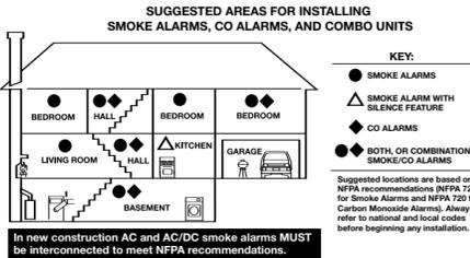
In new construction, AC and A/CO smoke alarms MUST be interconnected to meet NFPA recommendations.
