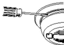
2. Pry the Smoke Alarm away from the bracket by turning both the screwdriver and the Smoke Alarm counterclockwise (left) at the same time.
