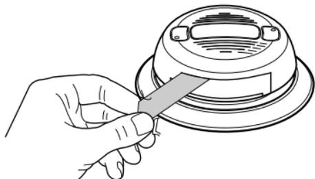
When the battery is activated, the red light will shine continuously for 5-10 seconds, then begin to flash about once a minute.
