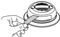
If the unit does not alarm during testing, DO NOT lock the battery compartment! Install a new battery and test again. If the Smoke Alarm still does not alarm, replace it immediately.
