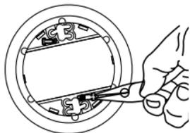
2. Insert the locking pin into the lock located on the pivoting hinge of the battery door.
