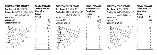
**CBCP** · Centerbeam candlepower **FC** · Footcandles at beam center (aim point)
