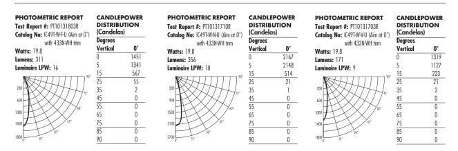
$\begin{array}{l} \textbf{CBCP} \boldsymbol{\cdot} \text{ Centerbeam candlepower} \\ \textbf{FC} \boldsymbol{\cdot} \text{ Footcandles at beam center (aim point)} \end{array}$
