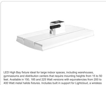
Project: Type: Prepared By: Date: **Driver Info** LED Info Type: Constant Current Watts: 185W 120V: 1.60A Color Temp: 4000K 208V: 0.92A Color Accuracy: 85 CRI 240V: 0.80A L70 Lifespan: 100000 277V: 0.69A 19865 Lumens: Input Watts: 180W Efficacy: 111 LPW Efficiency: N/A
