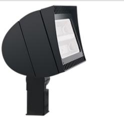
High power, wide distribution LED floodlight. Replaces 250W MH. Patent Pending airflow technology ensures long LED and driver lifespan. Use for building facade lighting, sign lighting, LED landscape lighting and instant-on security lighting.
