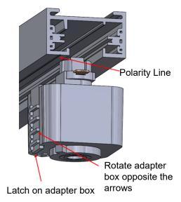
Rotate the adapter box opposite the arrows until the latch snaps in place between the two track rails
