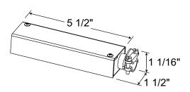
Note: Fully loaded run lengths longer than 18' with 12 AWG is not recommended due to voltage drop.
