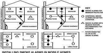
For minimum security install one Smoke Alarm as close to each sleeping area as possible. For more security, put one unit in each room. Many older mobile homes (especially those built before 1978) have little or no insulation. If your mobile home is not well insulated, or if you are unsure of the amount of insulation, it is important to install units on inside walls only. Smoke Alarms should be installed where temperatures normally remain between 40° F (4° C) and 100° F (38° C).
