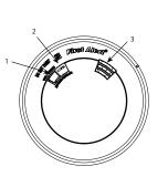
and Alarm indicator: Green LED provides visual indication of an Alarm Memory condition; Red LED provides visual indication of an Alarm and Hush modes 3 Speaker
