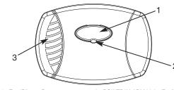
2 POWER/ALARM Light (Red) 1 Test/Silence Button 3 (Behind Cover) Alarm Horn: 85 dB audible alarm
