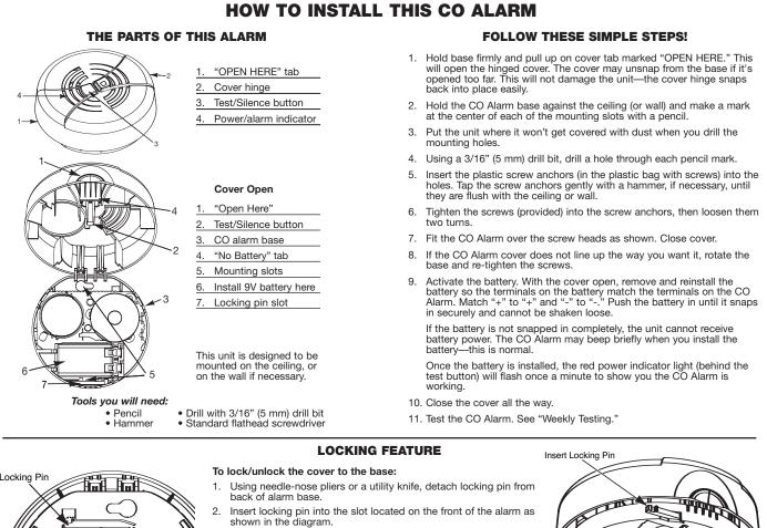
2. Insert locking pin into the slot located on the front of the alarm as
