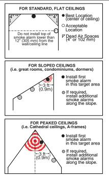
"Dead air" spaces may prevent smoke from reaching the Smoke Alarm. To avoid dead air spaces, follow the installation recommendations below.
