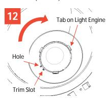
Align the opening in the trim with the tabs on the light engine. Rotate the trim clockwise until trim slot aligns with the hole in the trim holder. Secure trim with provided screw. Push the light engine up so it flush with the ceiling.
