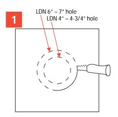
Cut ceiling opening slightly larger than the outside diameter on the mounting frame. 4" Ceiling opening: 4-3/4" (12.1cm). 6" Ceiling opening: 7" (17.8cm)
