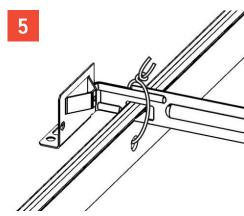
Secure channel bars to T-bar by means of wire ties.
