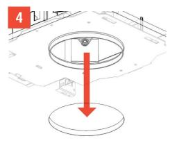
Position mounting frame through opening in ceiling.
