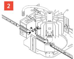
Assemble the channel bars to each side of the of the mounting frame with the included hardware. Leave the hardware loose to adjust the position of the frame in the ceiling.
