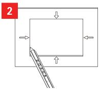
Using the square template, sketch the hole on the ceiling.
