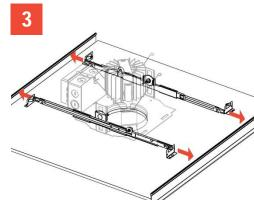
Adjust channel bars to the correct spacing between T-bar. See Page 4 for procedure for non-accessible ceiling installation.
