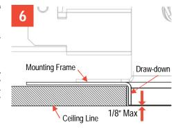
Adjust the mounting frame vertically to align the bottom edge of the draw-down to either flush or slightly above (1/8" max) the ceiling line.
