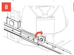
Re-tighten both channel bar clamping screws.
