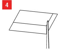
Using a keyhole saw, cut on sketched line. Return to section C-2 to complete the installation.
