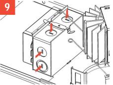
Remove knockouts on junction box to feed power supply to fixture. Supply wire must meet applicable electrical codes and be rated for a minimum of 90°C. Junction box is thru-wire rated for 8-No. 12 AWG conductors (4in-4out).
