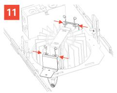
Squeeze wire springs on the light engine and insert each leg of the spring into the slots on the brackets on either side of the opening in the mounting frame. Pull the light engine down so the looped end of the wire spring rests on the top of the bracket.
