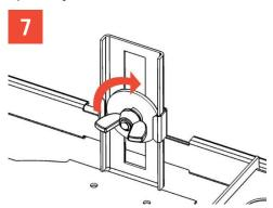
Re-tighten both vertical adjustment nuts.
