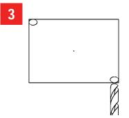
Drill a small hole at two corners of the sketched template.
