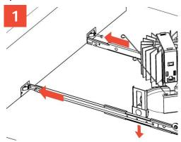
Mount to joists with flanges on channel bars resting against the bottom faces of the joists. Drive included nail into joist to secure. Move vertical adjustment to lowest point.
