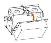
Complete necessary splices. Snap the door/driver assembly onto the junction box.
